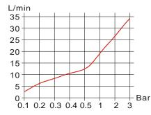
Test pressure: 1.6MPa (16bar) Flow pressure: Min 0.05MPa Max 1.60MPa Recommended pressure: 0.1MPa to 0.8MPa (1 to 8 bar)
